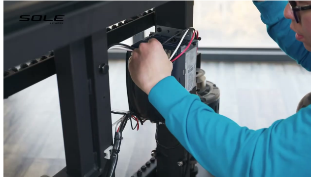
Motor control board (MCB) and wiring harness in the motor compartment.
