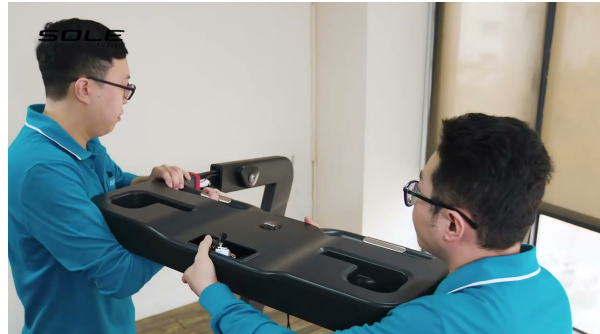
Console panel disconnected and lifted free.
