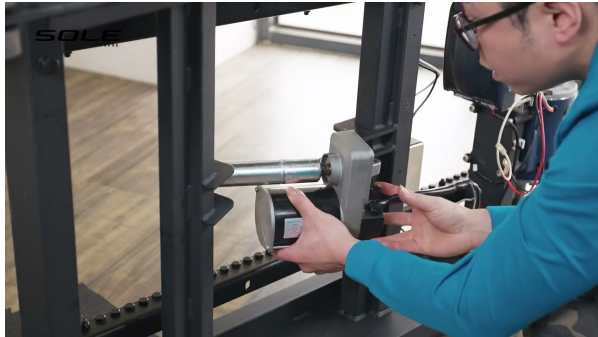
Incline motor/actuator being seated in the mast.
