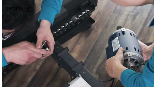
Drive motor removed from its mount.
