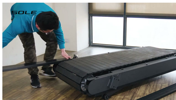
Tension released, slat belt coming off the rear roller.
