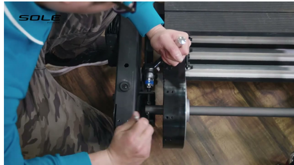
Removing the rear roller end bracket bolt.
